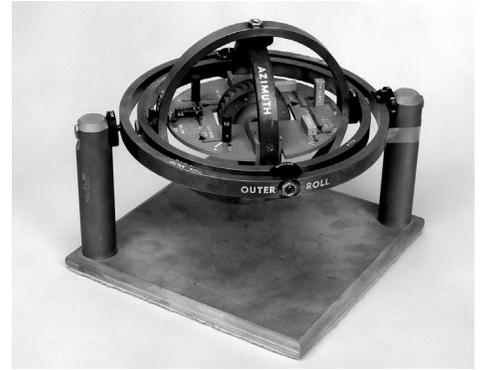
The gyroscope from an X-15 aircraft, to measure its position in three dimensions. Credit: NASA.
