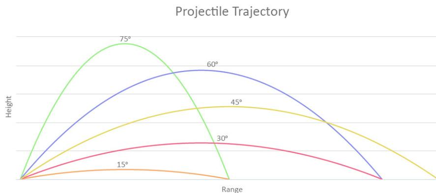
Distance of a projectile launched at different angles. Launch speed is the same in each case. A launch angle of  $45^\circ$  provides the longest flight for a projectile. Credit: Carnegie Science Center.
