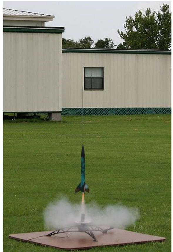
Model rockets use fins to stabilize their flight. Without fins, these rockets would easily tumble and fly off course.
