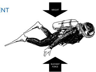
This diagram shows the direction of the buoyant force and weight (gravity) on a diver. Neutral buoyancy depends on balancing these two forces. Public domain image from Pearson Scott Foresman.
