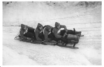
between the bobsled and the track? Early bobsleds were similar to wooden sleds used by children. The pilot steers the metal runners in front, and the person in the rear operates the brakes. Credit: German Federal Archive.
