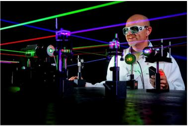
Calibrating range finders for the US Navy. Laser range finders are used to calculate the distance to an object and in 3-D modeling. Credit: US Navy photo by Greg Vojtko.
