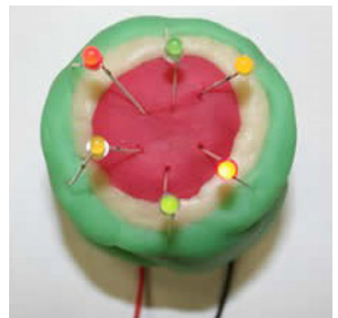
Conductive dough (red and green) and insulating dough (white) used to make a parallel circuit. Credit: University of St. Thomas.
